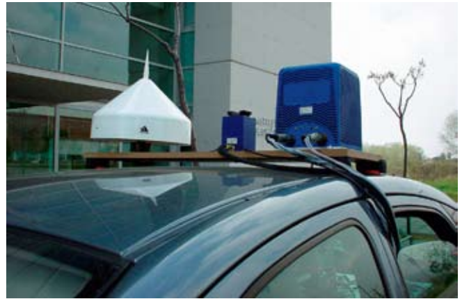
FIGURE 4 Data acquisition hardware configuration. From left to right: GPS precision antenna, automotive grade IMU, and navigation grade IMU
