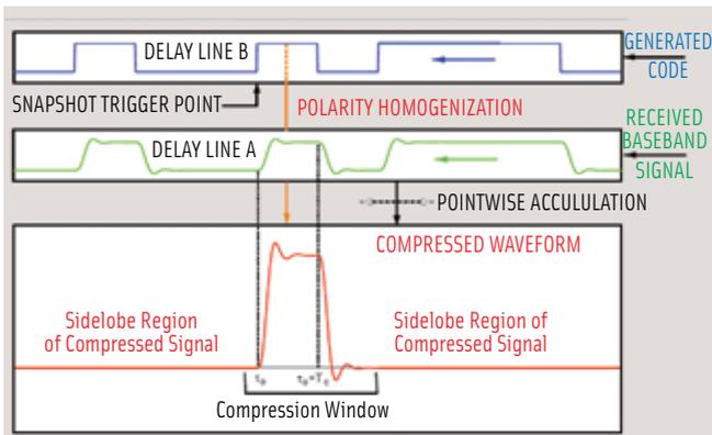
FIGURE 1 Visualization of signal compression
