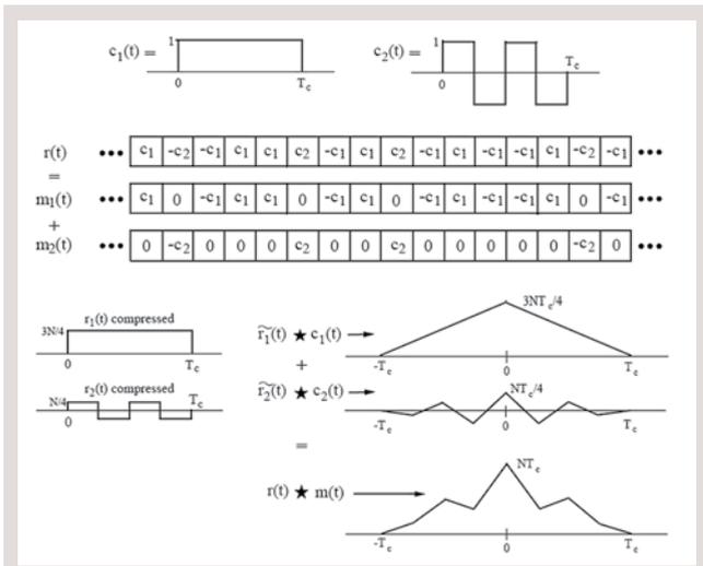
FIGURE 4 Compression of a TCMOC(2,1,1/4) signal
