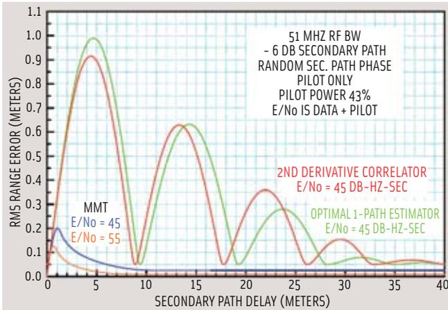
FIGURE 11 E5ab MMT comparative range error
