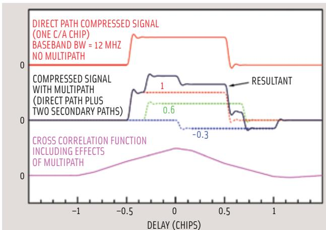
FIGURE 8 Extraction of multipath parameters
