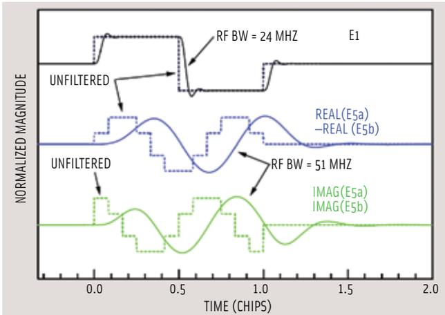
FIGURE 9 E1 and E5 compressed baseband signals
