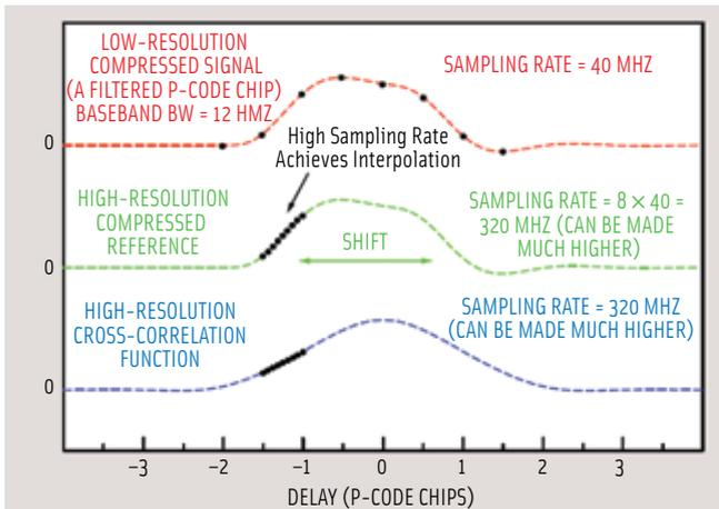
FIGURE 6 Computation of high-resolution cross-correlation functions
