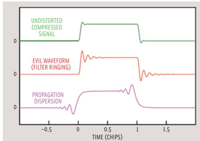
FIGURE 7 Observation of waveform anomalies
