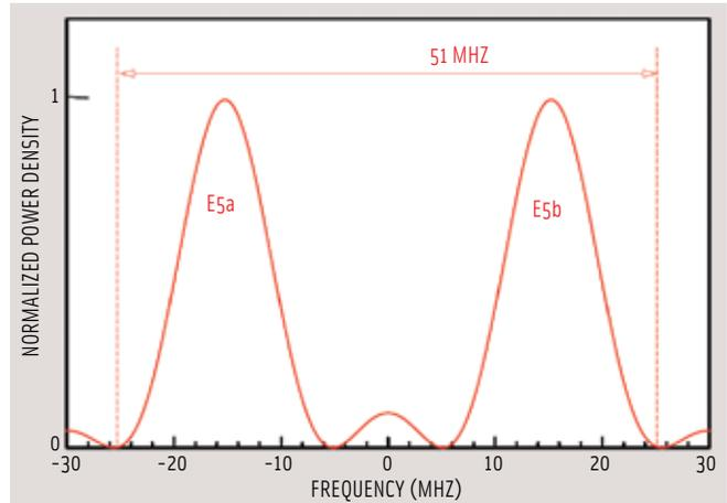
FIGURE 10 E5ab baseband power spectral density
