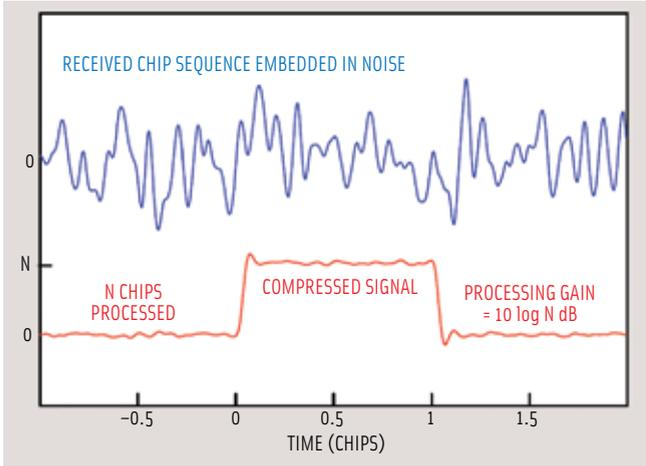
FIGURE 3 C/A-code signal visibility via processing gain
