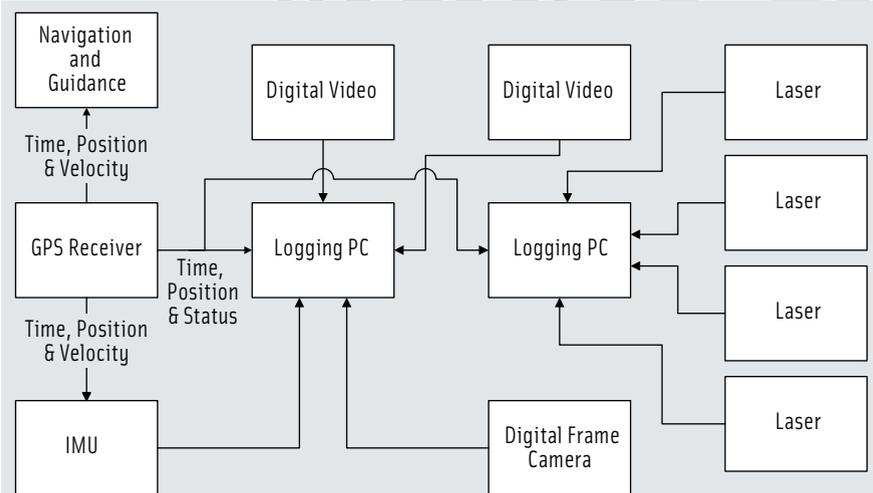
FIGURE 1 Block Diagram of TITAN System
