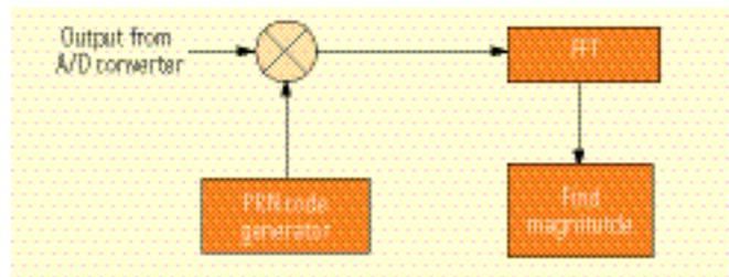
FIGURE 3 Parallel Frequency Search Receiver Architecture
