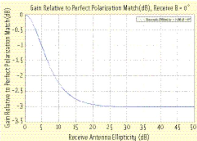
FIGURE 2 Losses Due To Ellipticity Assuming A Perfect Satellite Antenna
