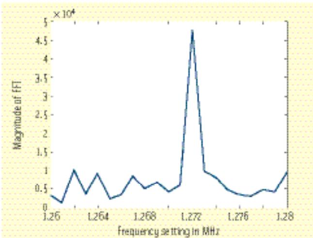
FIGURE 4 Doppler Frequency Determination using Parallel Frequency Search Approach
