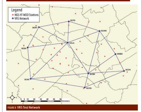
repeated a third time collecting a fivesecond data set at 1Hz. The data were recorded as a single-point value for each observation period using the South Carolina State Plane Coordinate System on NAD83/2007 and NAVD 88 for the orthometric heights. Accuracy Metrics. The design specification accuracy is just one component of the total system accuracy. The system accuracy must also include an estimate for the geodetic network accuracy and potential eccentricity of the rover over the survey mark.
