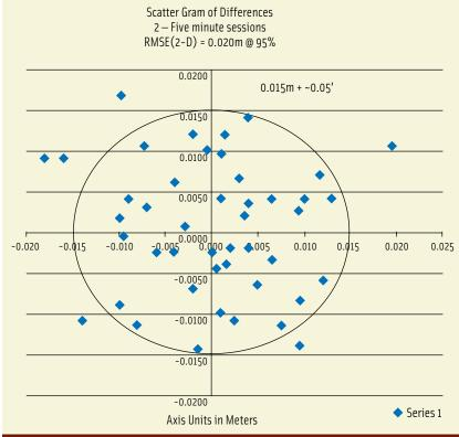
FIGURE 7 VRS real-time accuracy at the rover location of 1.2-centimeter (2-D RMSE)
