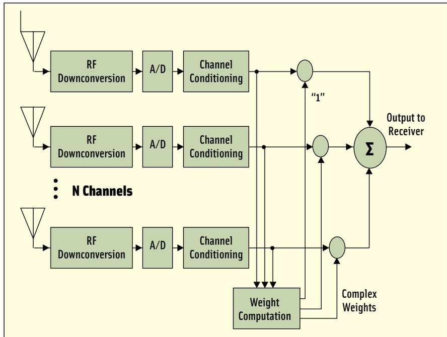
FIGURE 1 Single Output Nuller
