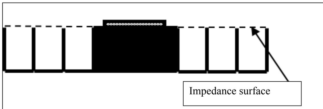
Fig.2 Cross-sectional view of the choke grooves structure of the original Choke Ring antenna with the impedance surface shown by dashed line.
