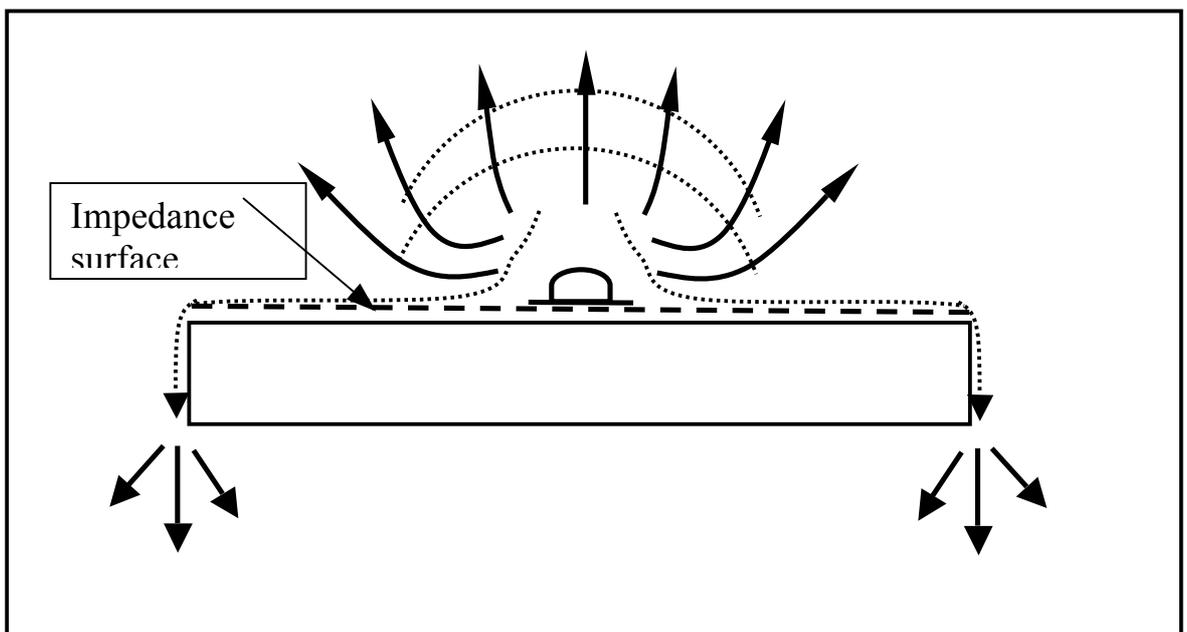
Fig.4 To mechanism of multipath rejection and antenna pattern narrowing with flat impedance structure.
