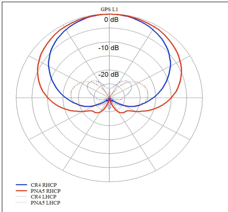
Fig8. Normalized antenna gain pattern for L1 frequency
