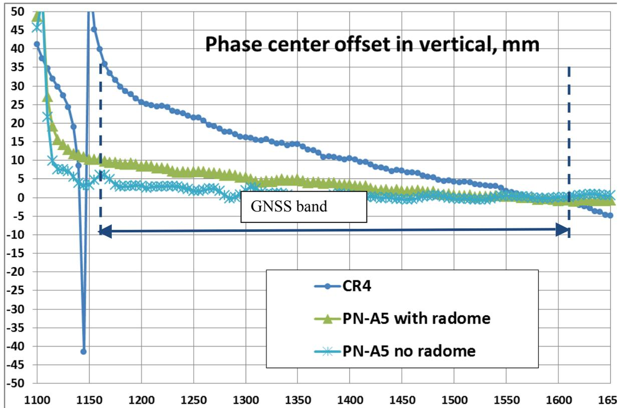
Fig.7 Phase center offset in vertical versus frequency of radiosignal.
