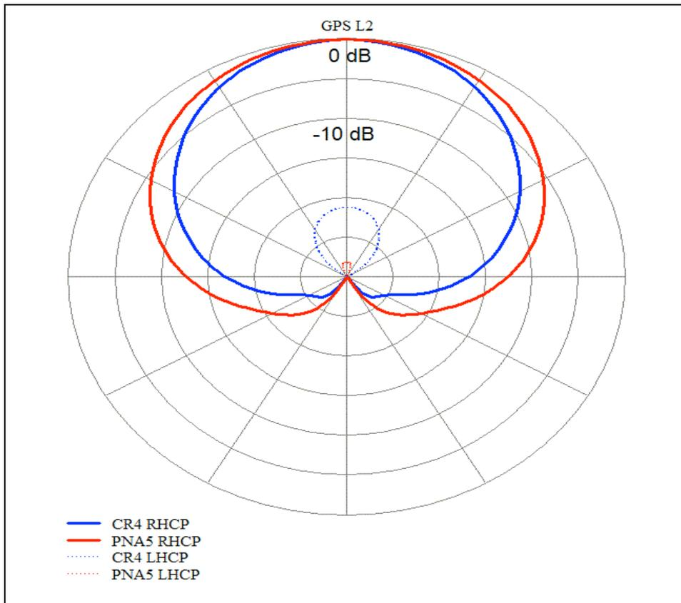
Fig9. Normalized antenna gain pattern for L2 frequency
