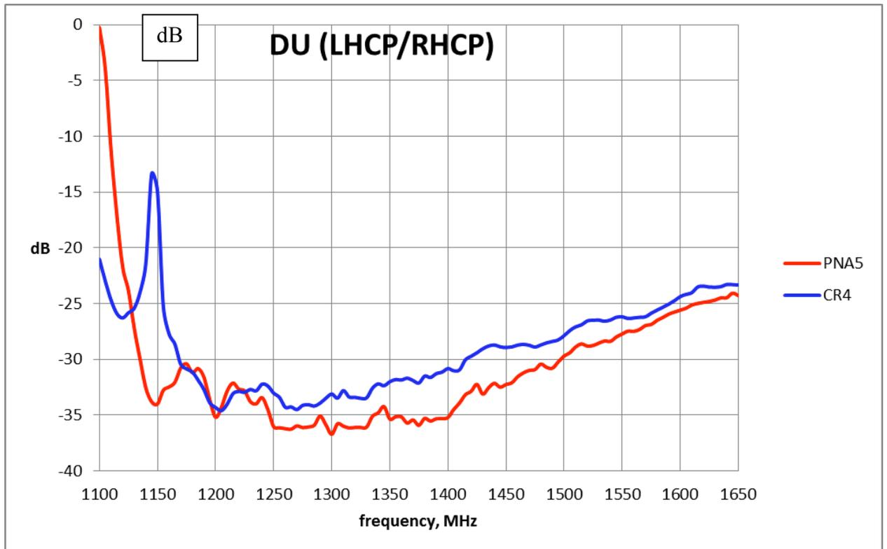
Fig.14 DU plot for zenith direction versus frequency.
