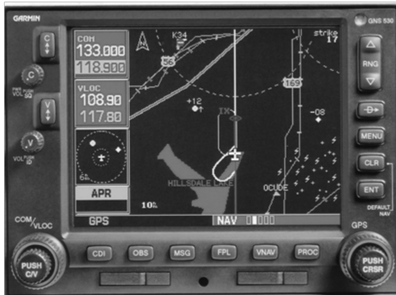
Figure 6. Panel Mount General Aviation GPS Receiver, approximately 6.25 in × 4.60 in × 11.0 in, 9.5 lbs (courtesy of Garmin)
