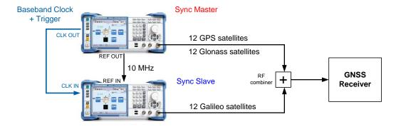
One SMBV acts as master instrument and supplies all necessary synchronization signals to the slave instrument via just two connection cables. The instrument setup is simple, easy to configure and provides highly synchronized signals. It is explained in more detail in reference [2].
