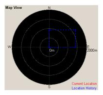
The position reported by the receiver is compared with the simulated position defined in the waypoint file. A 2D and 3D position error is calculated by calculating the distance between the reported values for longitude, latitude and altitude and the defined values in the waypoint file. For testing, the reference level is usually set to a level well above the acquisition sensitivity level of the receiver.
