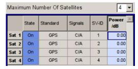
In this example, each satellite signal will have a level of –130 dBm, and four satellites together will have a level of four times –130 dBm, which equals –124 dBm [4].
