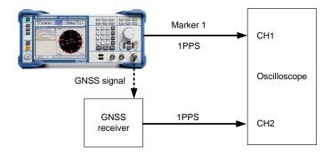
By measuring the time difference between the pulse edges of the two 1PPS signals over a period of time, the pulse stability or jitter can be determined. The precision of the receiver's 1PPS signal is related to the time dilution of precision (TDOP) of the satellite constellation.
