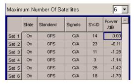
The displayed power offsets in the satellite configuration table correspond to the values at the start of the simulation. Note that these displayed values are not updated, although the power offsets change automatically during the simulation.
